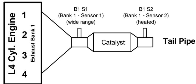
Figure 12: Schematic diagram of oxygen sensor arrangement
