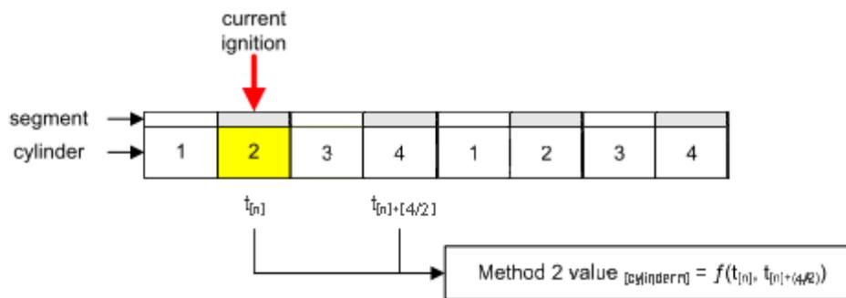
Figure 7: The second method of misfire monitoring
