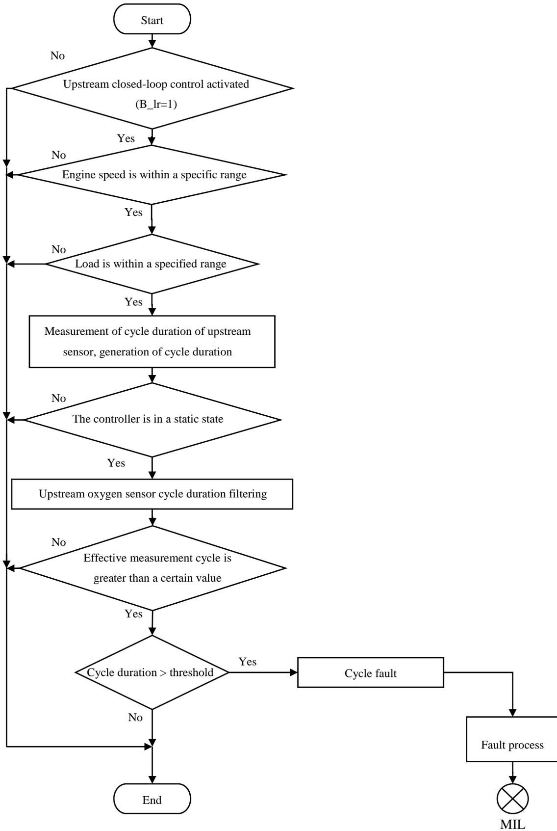
Figure 13: Monitoring process of periodic aging of oxygen sensor
