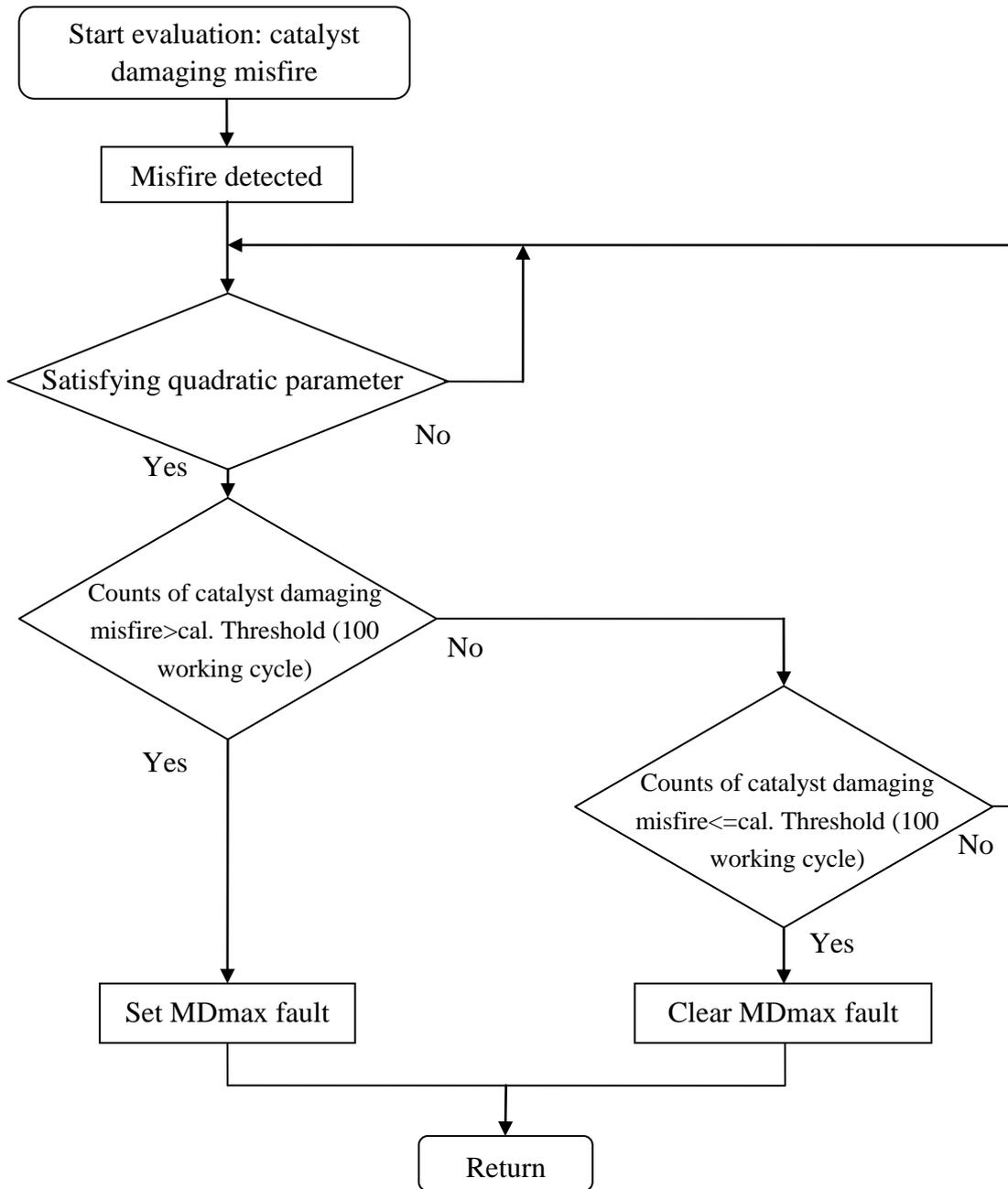
Figure 11: Misfire monitoring - subprogram "damage catalyst monitoring"
