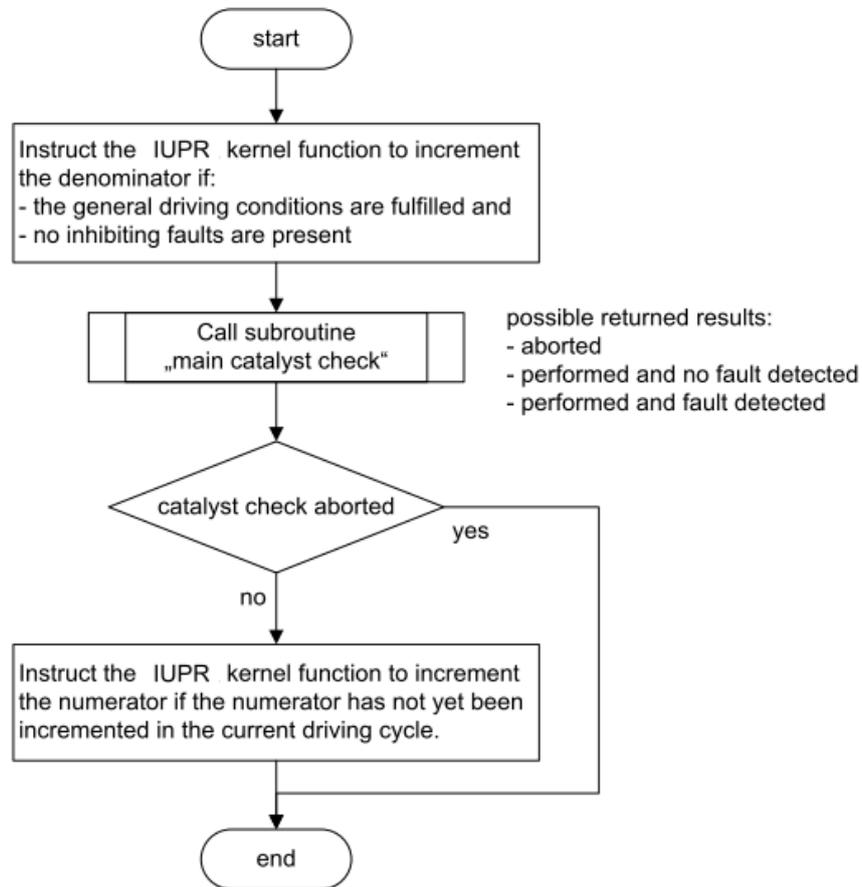
Figure 3: Aging monitoring of catalytic converters-main flowchart
