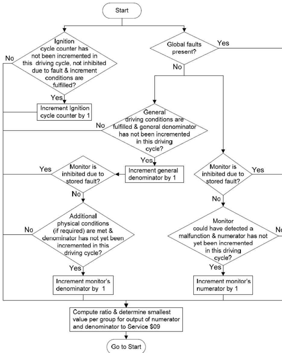
Figure 15: Minimum diagnostic rate flowchart
