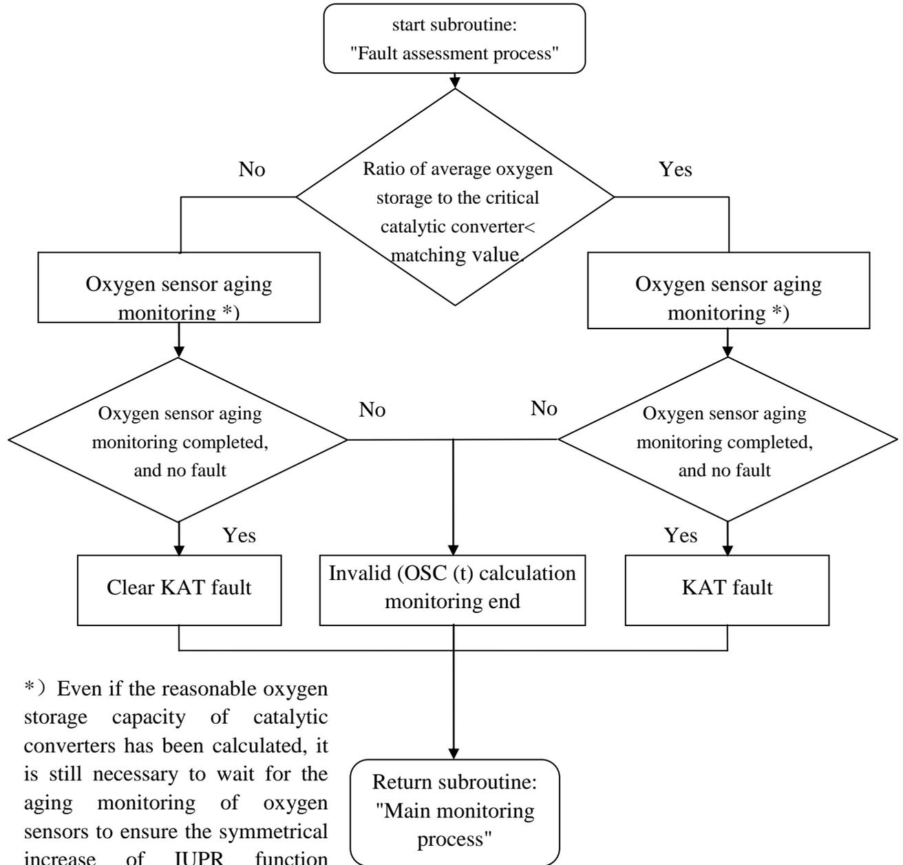
Figure 5: Catalyst monitor – subroutine “error evaluation”
