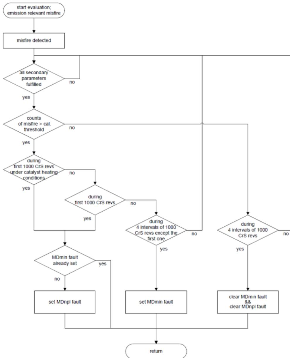
Figure 10: Misfire monitoring --subprogram "emission deterioration misfire monitoring"
