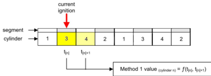
Figure 6: The first method of misfire monitoring
