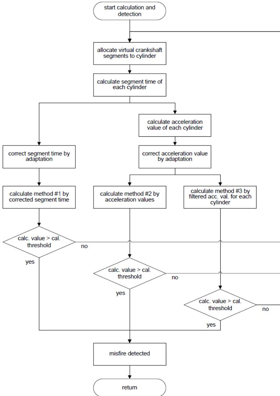
Figure 9: Misfire monitoring - subroutine "calculation and monitoring"
